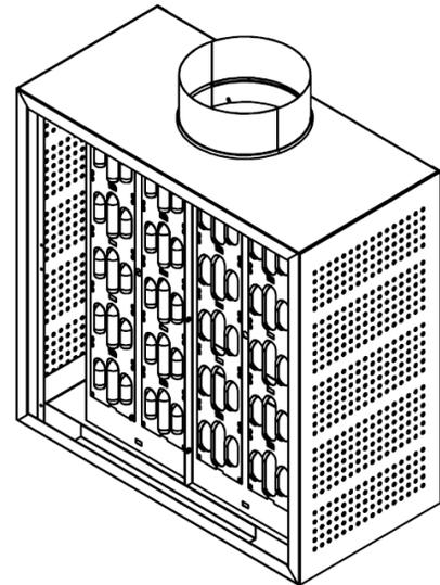
View showing integral variable air pattern controllers
